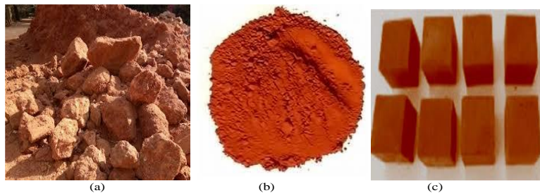
Figure 5a. widely utilized RM raw (natural) materials; a) raw; b) Powder form; c) made with RH geopolymer.
