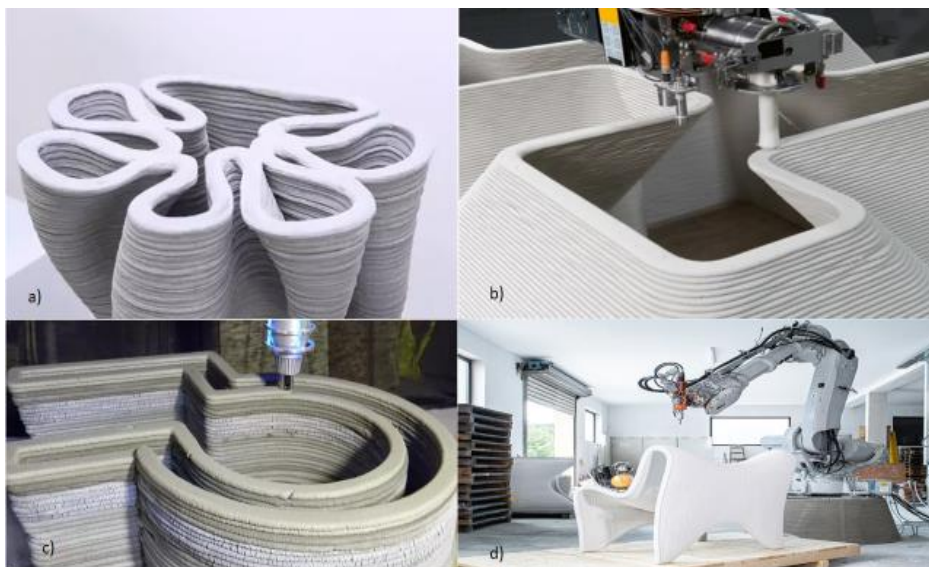
Figure 3. Geometric freedom of complex structures using 3D concrete printer (a, source:www.sculpteo.com), (b, source:www.googleimages.com), (c, source: www.sculpteo.com) and (d, source:googleimages.com).
