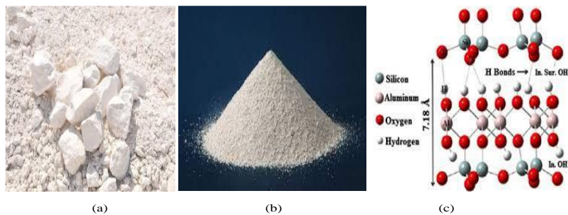
Figure 6a. widely utilized MK raw (natural) materials; a) raw; b) Powder form; c) Bonds
